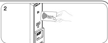
Present the RFID credential to the RFID reader.
