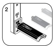
While the LED is flashing, insert one Manager Key at a time. A two-tone beep will be heard for each Manager Key programmed.
